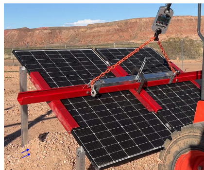
PHOTO 8: Test 2 - Evidence of ballast shift
