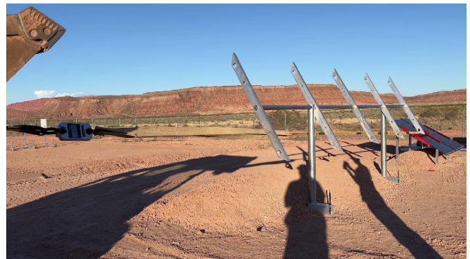
Photo 4: Horizontal force test at max load
